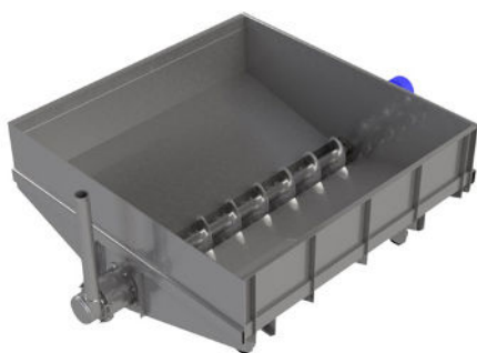
Ground Meat is Metered and Pumped for Further Processing
