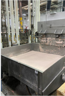
Ground Meat Mixture is Captured by Hopper and Fed to Pump
