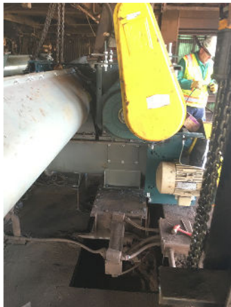
New Screw Conveyors Fit in Very Limited Space
