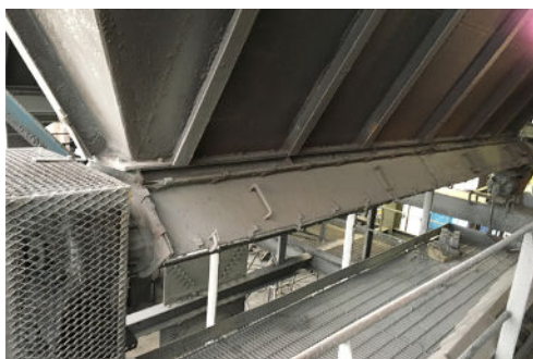
Old Equipment was Replaced with Heavy-Duty KWS Screw Conveyors
