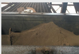
Electric Arc Furnace (EAF) Dust is Extremely Dense and Abrasive
