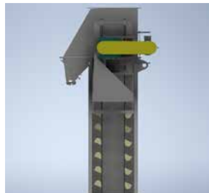
Head Section Take Up Allows Close Clearance Clean Out in Boot Section
