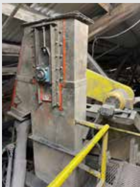
CertainTeed Added a Clean-Out Door to Existing Bucket Elevator to Clean Out Boot Section
