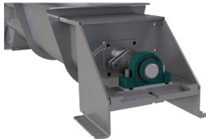
Slider Base Trough End Allows Axial Thermal Expansion
