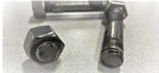
Coupling Bolt Failure Due to Screw Conveyor Misalignment and Excessive Vibration
