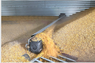
Grain is Swept to Openings in Bottom of Bin and Removed with Floor Auger
