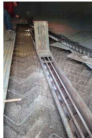
New KWS Floor Auger Receives Grain from Sweep Auger and Removes it from Bin
