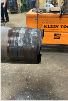
Existing Screw Failed Due to Corrosion and Wear
