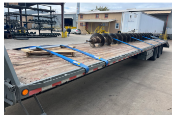
Completed New Drive Shaft and Repaired Screw on Hot Shot Back to Georgia Pacific Plant
