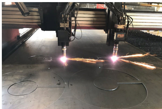
Flights are Cut on High Definition Burn Table to Exact Dimensions
