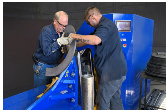
Flights are Formed Using Special Forming Machine
