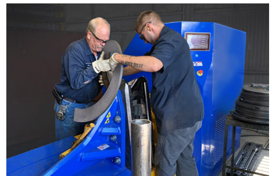
Flights are Formed Using Special Forming Machine
