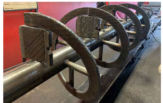
Center Drive Shaft is 7-Inch Diameter Solid Bar with 1-1/2-Inch Diameter Posts for Mounting 1-Inch Thick Ribbon Flighting
