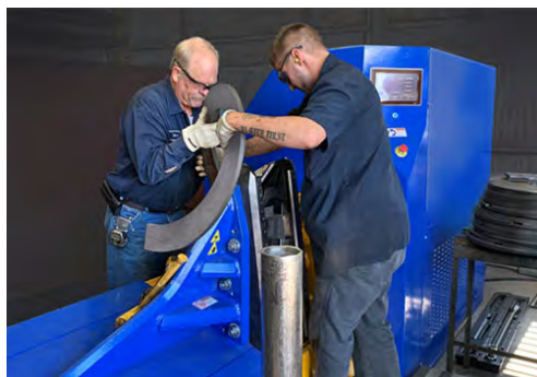
Flights are Formed Accurately on Special CNC Machine
