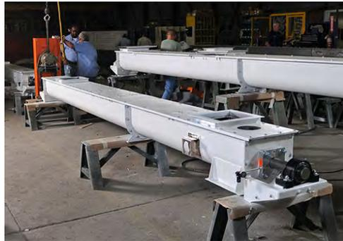
KWS Provides Heavy-Duty Screw Conveyors
