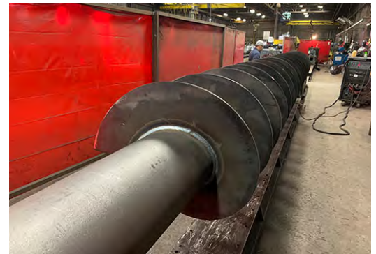
New KWS Screw is Mounted on Large Diameter Pipe with Continuous Welds
