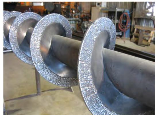
Hardsurfacing is Applied to Carrying Face and Outer Edges of Screw Flights
