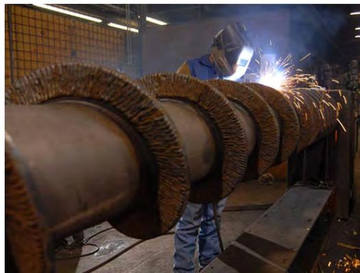
KWS Welder Applies Weld-On Hardsurfacing to Screw Flights for Wear Resistance
