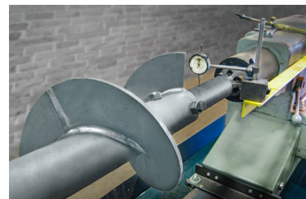
KWS Screws are Straightened to Within 0.015-Inches TIR
