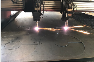
Sectional Flights are Cut on High Definition Dual-Head Plasma Table for Maximum Efficiency
