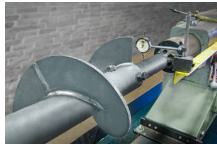
KWS Screws are Straightened to Within 0.015-Inches TIR
