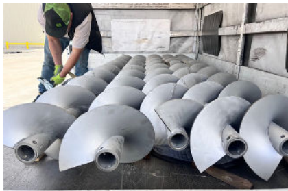
Stainless Steel Screws are Loaded in Hot Shot for Direct Delivery to PPP Plant
