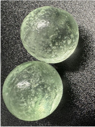
Glass Spheres are Extremely Abrasive and Difficult to Convey
