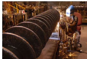
Carrying Faces, OD, and Center Pipe are Hardsurfaced with Chromium Carbide
