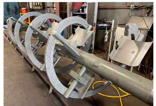
KWS Designed the New Screws for Maximum Mixing and Wear Resistance
