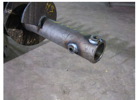
New KWS Screw is Stronger with Schedule 80 Pipe and Bolt Pads
