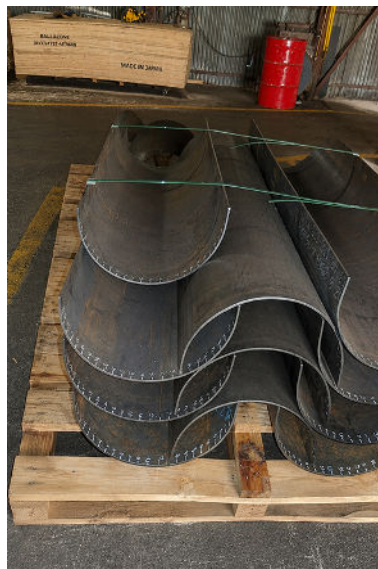
Eleven AR235 Abrasion Resistant Trough Liners Delivered to Site
