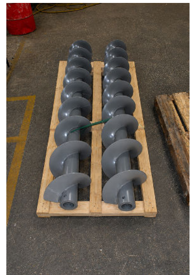
Heavy Duty Screws Mounted on 5-Inch Schedule 120 Pipe
