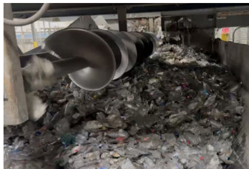
Leveling Screws Provide Consistent Material Distribution
