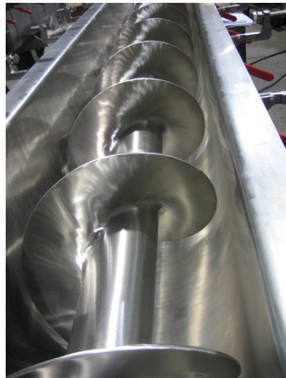
KWS 304 Stainless Steel Screw Conveyor Conveys Citrus Pulp
