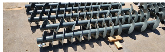
Both Left-Hand and Right-Hand Screws with Abrasion-Resistant Flights were Required
