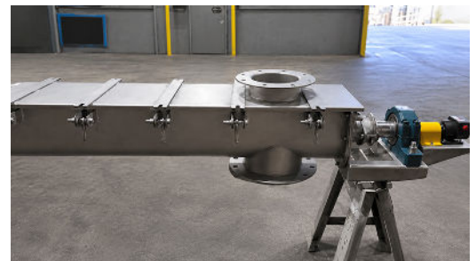
Screw Conveyor Holds Internal Pressure
