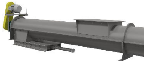
Design Upgrades Included Split Tubular Troughs and a New Drive Unit
