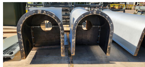
Special Baffles Prevent Hot Material from Migrating to Shafts
