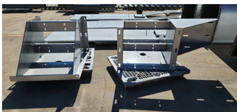
Pedestal Trough Ends are Painted High Temperature Silver and Ready for Shipment
