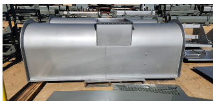
Troughs are Oversized for Installation of Refractory Lining
