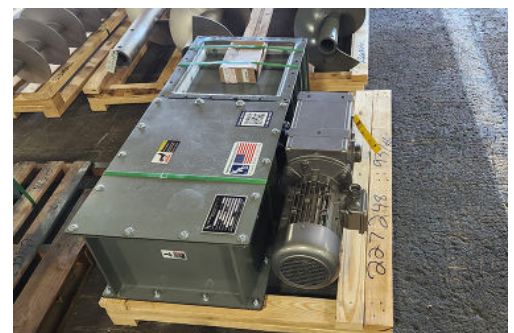
High-Torque Drive Unit Generates Sufficient Force for Opening and Closing Under Load
