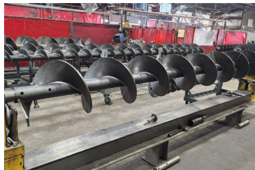
KWS Upgraded Screw Construction to Significantly Increase Rigidity and Eliminate Failure
