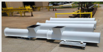
Screw Conveyor Components are Painted White in Accordance with Nestle Standards
