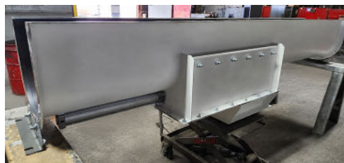
Pneumatic Actuators Power Curved Slide Gates
