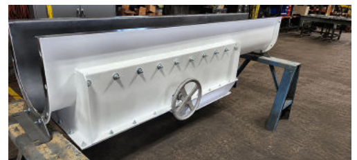
Hand Operated Curved Slide Gate is Used in Tight Location
