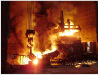
Electric Arc Furnace (EAF) Method Converts Recycled Metals into Steel
