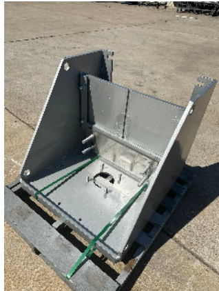
Slider Base Allows for Axial Thermal Expansion
