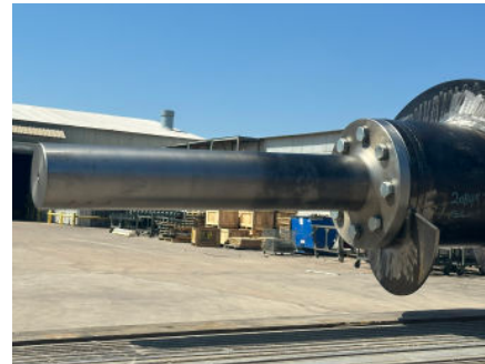
Flanged Tail Shaft is Bolted to Screw Assembly
