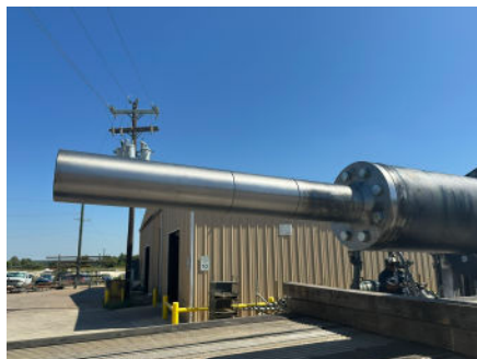
Flanged Drive and Tail Shafts are Machined from Single Piece of Bar Stock and Will Not Fail
