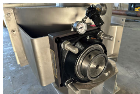
Seals and Bearings are Mounted on Outside of Trough End
