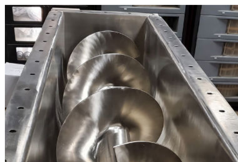
Studs are Welded, Ground Smooth, and Polished on Inside of Trough End
