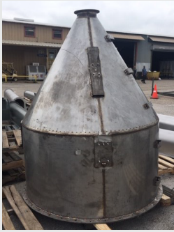
Hopper Before Passivation with Impurities, Stains, and Scale
