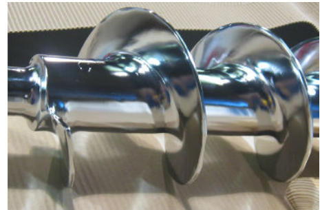
Electropolished Screw Surfaces are Smooth and Shiny
