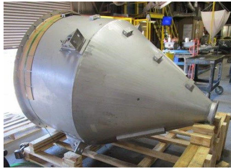
Hopper After Passivation with Impurities Removed and Clean Finish
