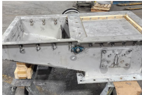
Pickling Removes Weld Scale and Heat Tint and Leaves Dull Gray Matte Finish
