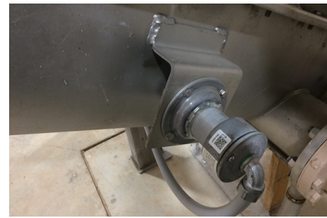
Mounting Bracket is Welded to Housing and Probe is Adjustable
