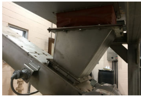
Milltronics MSP12 Inductive Probe Senses Rotating Shaftless Spiral of KWS Screw Conveyor
