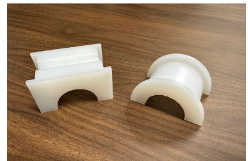
UHMW Hanger Bearings are Recommended for Light to Moderate Loads and Speeds Up to 60-rpm
