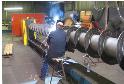
Special Hardsurfaced Screw was Manufactured and Delivered within 2 Days to Meet Customer Requirements
