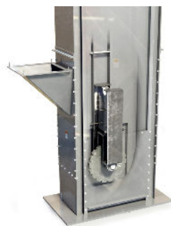
Internal Gravity Take Ups Automatically Maintain Chain or Belt Tension
