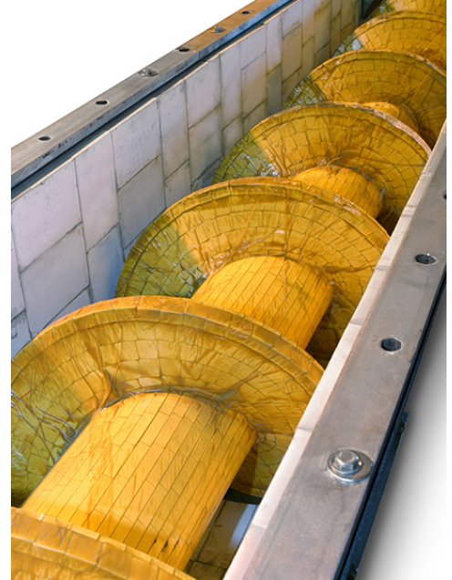
Extended Lifespan and Reduced Maintenance Make Ceramic Liners Cost-Effective for Demanding Applications
