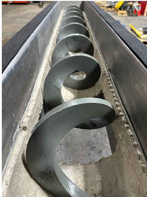
Alumina Silica Ceramic Tiles Provide Superior Hardness and Wear Resistance
