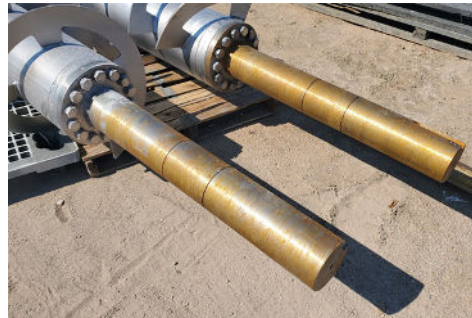
KWS Flanged Shaft-to-Pipe Connection Will Not Fail
