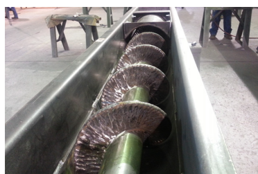
AR 400 Liner in Trough Provides Excellent Abrasion Resistance
