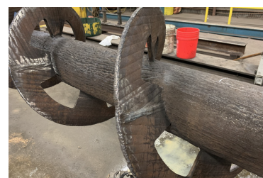
Chromium Carbide Overlay Plate is Used for Screws to Convey Glass Cullet and Alumina
