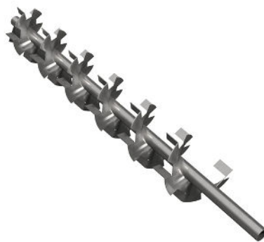
Outer Edge of Each Flight is Cut and Folded to Form Integral Lifting Paddles
