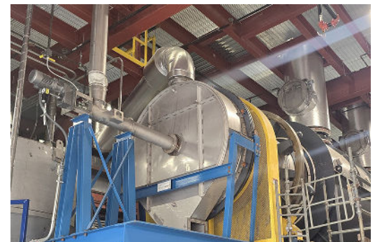
KWS Cantilevered Design Eliminates Tail End Bearings
