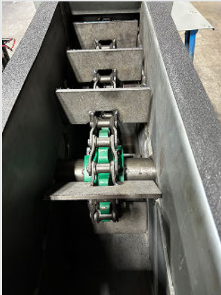
Welded Steel Chain is Constructed with Hardened Bushings and Pins
