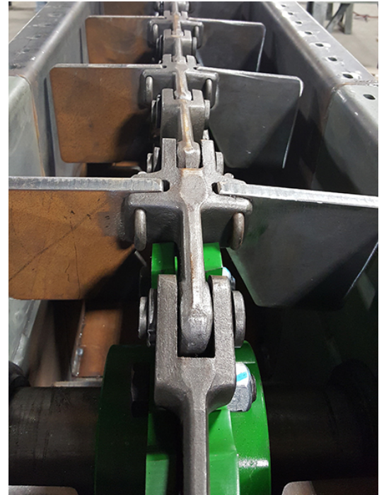
Drop-Forged Chain is Heat-Treated Alloy Steel Case-Hardened to Rockwell C57-C62
