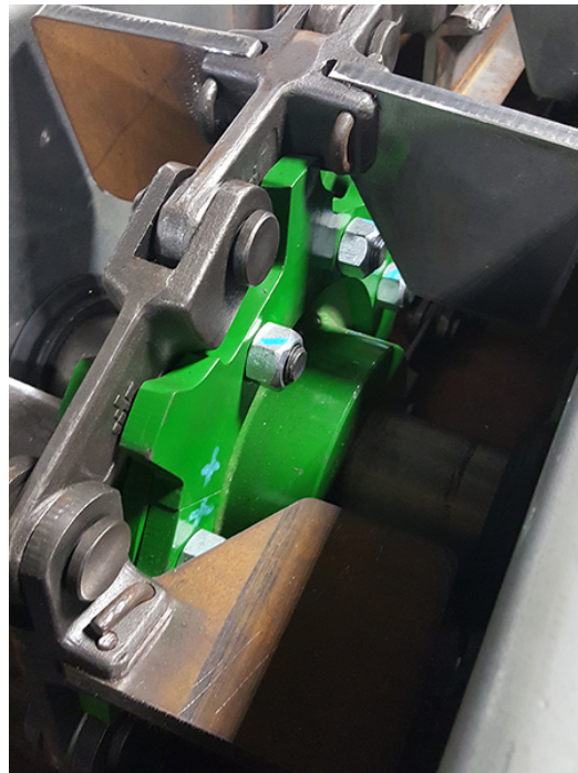
Split and Segmental Rim Sprockets Allow for Quick Replacement
