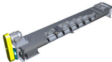
Screw Conveyors are Always Control Fed at Inlet
