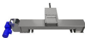
Control Valve Must Be Located Above Reversible Screw Feeder to Stop Bulk Material Flow Before Reversing Screw Feeder
