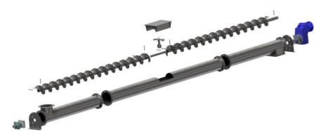
If your conveyor system has additional hanger pockets, follow the same procedure when designing the conveyor to ensure that all hanger pockets avoid trough flanges, and center all hanger pockets on a trough when possible.
