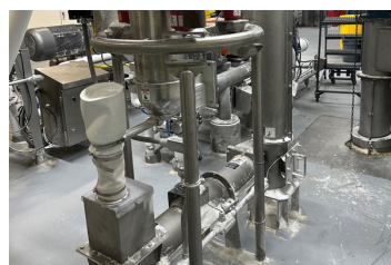
Inlet End is Supported by Securing Base to Floor
