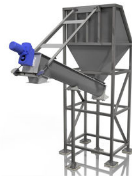
KWS Recommends an Inlet Length of No More Than 2 Times Diameter for Inclined Screw Feeders
