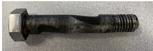
Shank of Coupling Bolt is Worn in Bearing Area Due to Repeated Starts and Stops of Vertical Screw Conveyor
