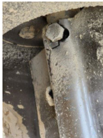
Repeated Stops and Starts Along with Improper Coupling Bolts Caused Screw Failure
