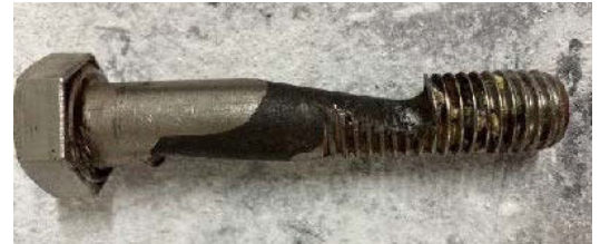
Use of Improper Coupling Bolts Contributed to Screw Failure
