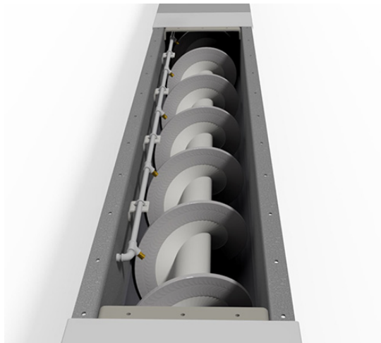
Spray Nozzle System Lightly Coats Screw Flights with Water to Reduce Chromium Paste from Sticking
